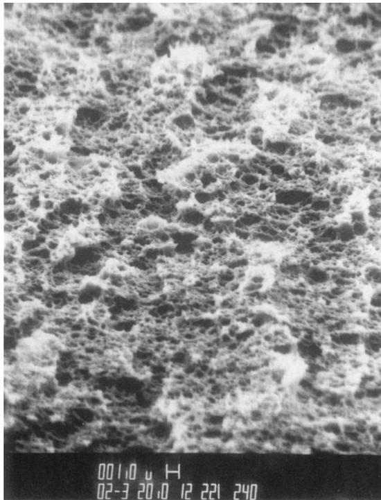
Fig. 7. SEM high magnification view of an ABS fracture surface taken near to an internal source. Sample tested at  $\dot{\epsilon} = 8.3 \times 10^{-4} \text{ s}^{-1}$ .
