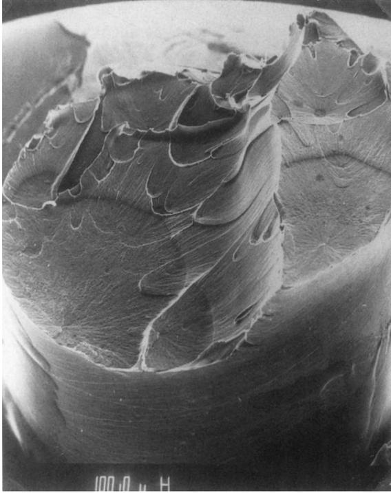
Fig. 14. SEM scan of the fatigue fracture of an ABS sample tested at 27.6 MPa and 0.2 Hz.
